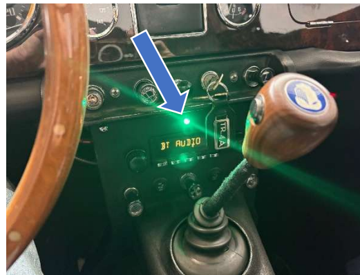
Figure 4c/ TR4-TR4A External LED location above radio
