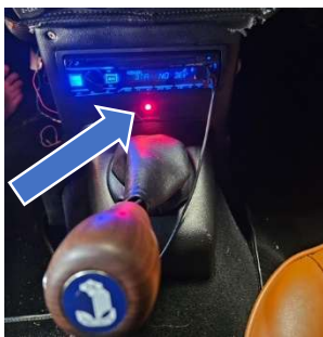
Figure 4b/ TR6 External LED Location under the radio
