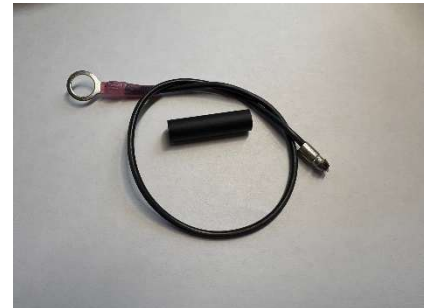
Figure W4/ Interrupt Switch Ground Wire
