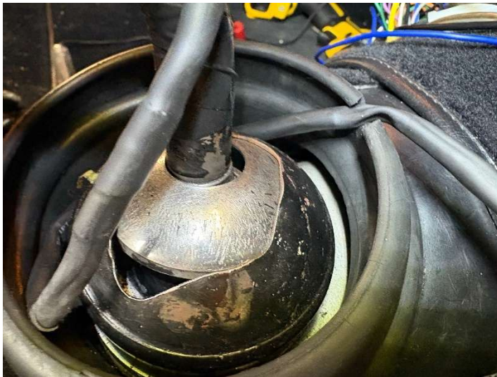
Figure 11/ top view of correctly routed cable
