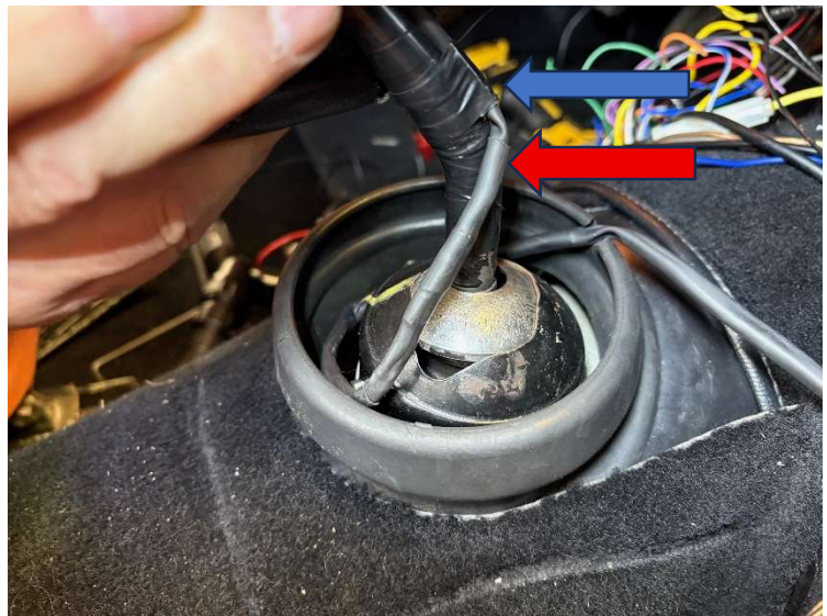
Figure 8/ shrink sleeving and cable restraint
