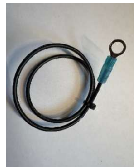
Figure W2/ Controller Ground Wire
